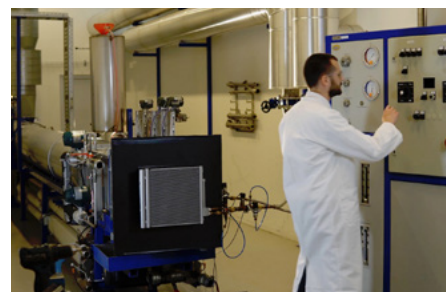
Nissens controls the superior condenser quality through various test series, including performance validation in the wind tunnel.
