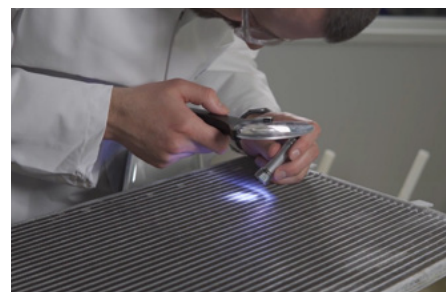
The 400-hour salt chamber corrosion test has proven that Nissens' condenser maintains its structure with no signs of corrosion.
