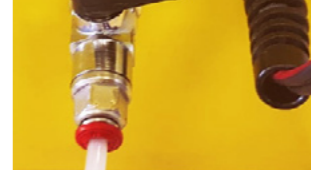
Closed supply valve of the MT424 equipment- Open it by pulling
