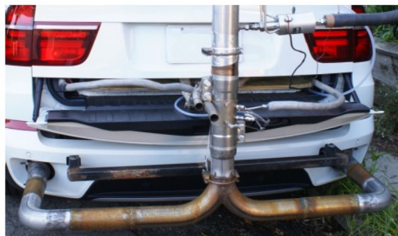
Figure 3.26: Exhaust adapter setup for Vehicle C, left : 3.5" exhaust flow meter (EFM), right : joining double vehicle exhaust stack into exhaust transfer pipe
