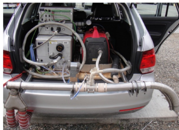
Figure 3.21: Vehicle A instrumentation setup
