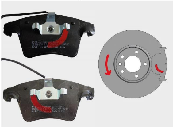
Caption 2: The curved cut-out on the backing plate is an indication of a directional brake pad.
