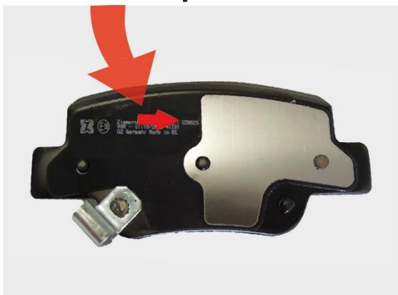
Caption 1: Arrows on the backing plate, which indicate the direction of rotation of the brake disc, serve as an aid for the correct installation of Zimmermann brake pads.
